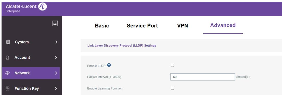
The screenshot shows the Alcatel-Lucent Enterprise Web UI. The left sidebar contains a navigation menu with 'System', 'Account', 'Network', and 'Function Key'. The main content area has tabs for 'Basic', 'Service Port', 'VPN', and 'Advanced'. Under the 'Advanced' tab, there is a section for 'Link Layer Discovery Protocol (LLDP) Settings'. This section includes three settings: 'Enable LLDP' (unchecked), 'Packet Interval: (1-3600)' (set to 60 seconds), and 'Enable Learning Function' (unchecked).
