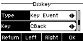
Figure 23 - Set the Callback key on the telephone
