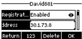
Figure 99 - SIP address and account information
